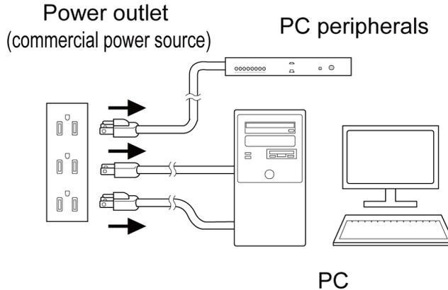
2. Connect the equipment requiring backup to the UPS's "power output" outlet.
