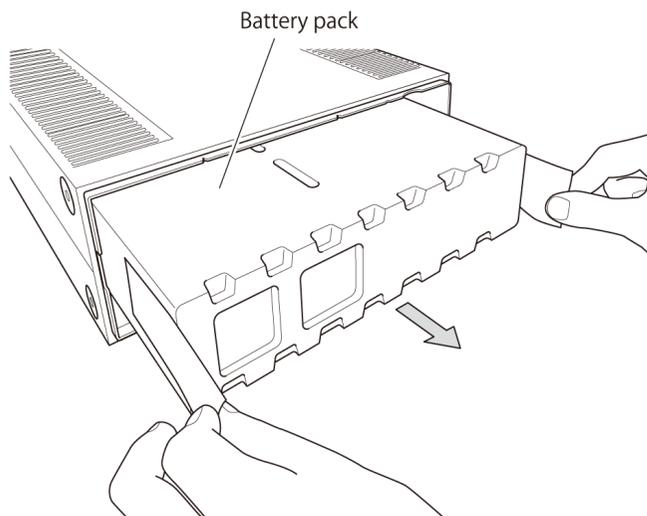
5. Insert the new battery pack. Securely push the battery pack until the connector on the rear of the battery pack is connected to the unit.
