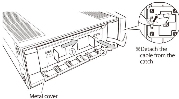
4. Remove the battery pack by pulling the tapes in its both sides.
