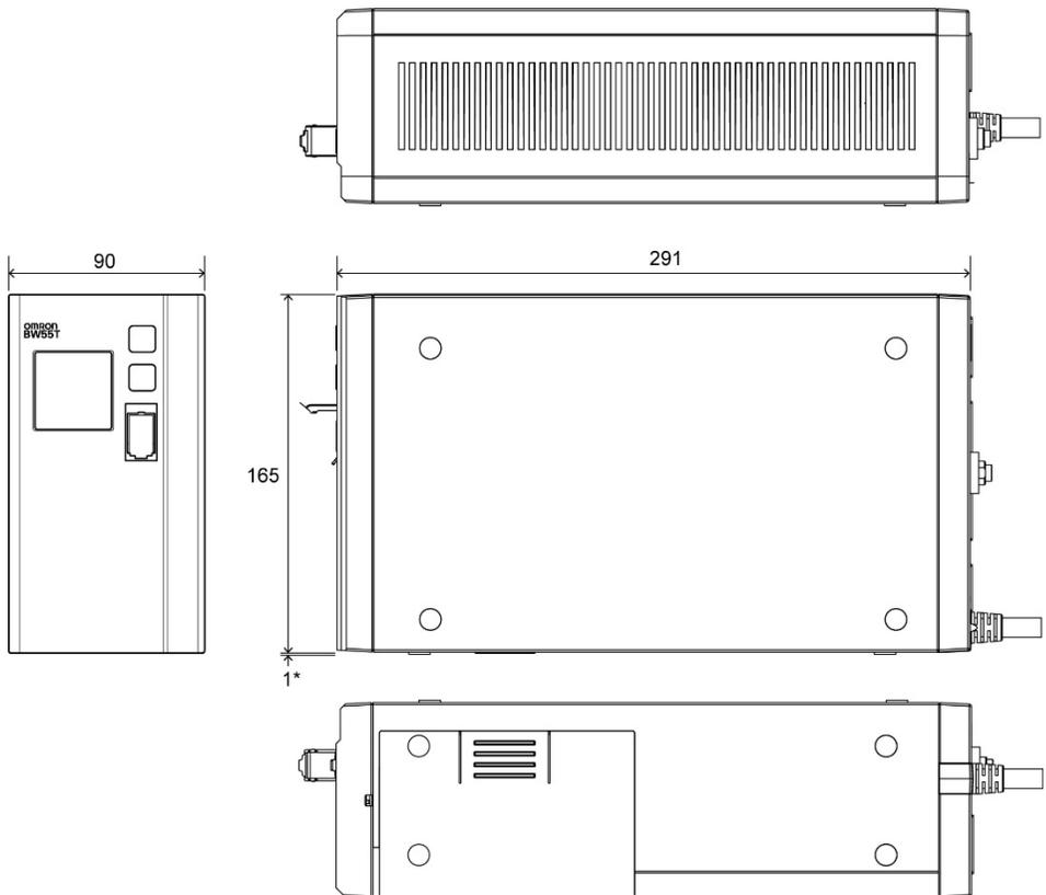
\* The thickness of rubber feet is 2 mm, but the main body has depressions, so the height is 1 mm.
