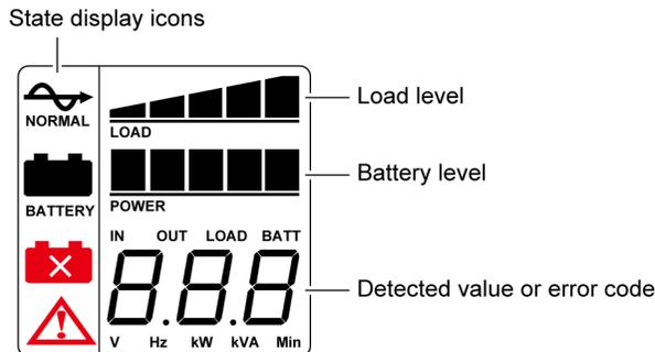
\* This screen shows "all lighted" state for explanation. When the display is turned off, it turns on again by pressing a button.
