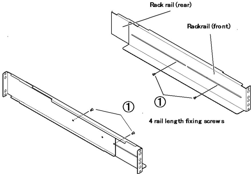
2. Adjust the length of support angles to suit the server rack, and then securely tighten the screws that were half-tightened in step 1. (②)
