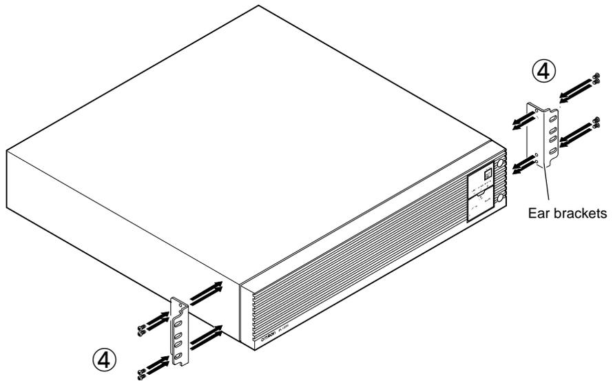
5. Place the UPS on the support angles and push it completely into the rack (⑤), and use the 2 included EIA/JIS rack fixing screws (M5) to securely fasten the ear brackets to the server rack. (⑥)
