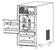
**4**. Hold the pullout label at the bottom of the upper battery pack and remove the battery pack.
