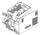
**4**. Hold the pullout label at the bottom of the battery pack and remove the battery pack.
