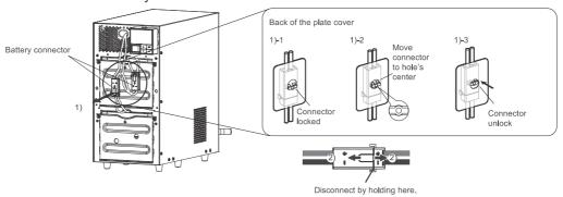
**3**. Turn the 2 screws that fix the plate cover over the upper battery counter-clockwise to remove them. 1)
