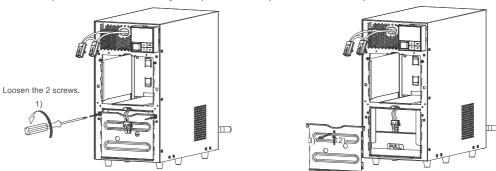
**6**. Hold the pullout label at the bottom of the lower battery pack and remove the battery pack.
