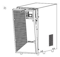
**2**. Remove the battery connector from the plate cover. 1)
