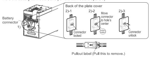
**3**. Turn the 2 screws that fix the plate cover counter-clockwise to remove them. 1) Pull the plate cover towards you 2) and lift it up to remove it. 3)
