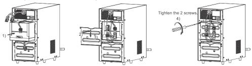
**9**. Insert the connector until it is locked. 1)
