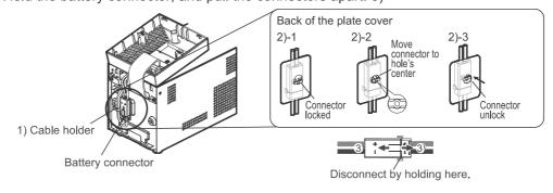
**3**. Turn the 2 screws that fix the plate cover counter-clockwise to remove them. 1) Pull the plate cover towards you 2) and lift it up to remove it.3)
