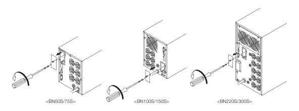
(2) Carefully insert the SNMP/Web card (model number: SC20G), and securely tighten the 2 screws. \* Replace with BU50SW/BU75SW/BU100SW/BU150SW/BU1002SW/BU3002SW brackets.
