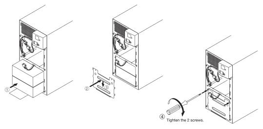
8. Insert a new battery into the UPS as far as it will go. ①● Replacement battery pack
