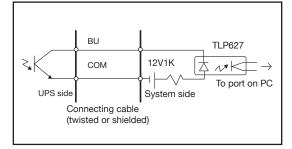
• Example of BS signal input circuit and the connected circuit
