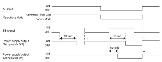
Note 1: Operation when setting switch 2 is OFF (auto startup is performed). When it is ON (auto startup is not performed) auto startup is not performed.
