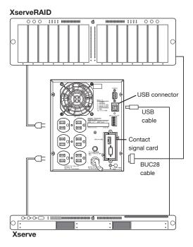
(6) Turn ON the power switches for the Xserve RAID and the UPS.
