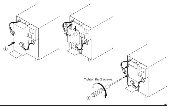
**6.** Insert the connector until it is locked. ①
